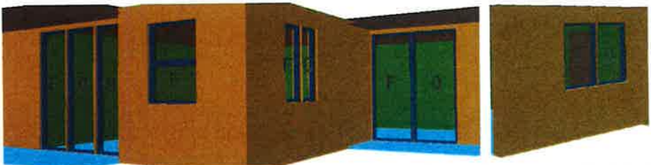
Figure 3: Aperture configuration - front of lightwell-connected apartment (left); lightwell-connected bedroom window (right); F denotes the fixed windows/doors | O denotes the operable windows/doors
